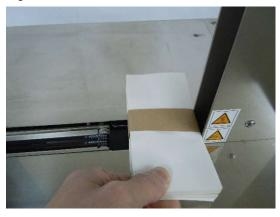
③ When an article is removed from the table, the next tape is automatically set on the arched guide.
