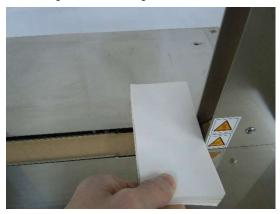
② Once the START switch is pressed, the tape is tightened, glued, and cut, and banding is completed.
