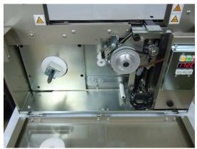
③ Place a tape on the paper tube holder. \*Be careful with the direction of the tape.
