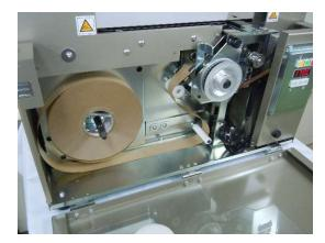
⑤ Insert the tape end into the tape guide, pass the tape until it touches the rubber roller, then lightly put a hand on the arrow, and hold the tape.
