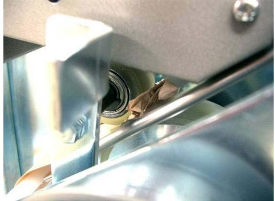
REMEDY : Remove the sticky material using a file.
