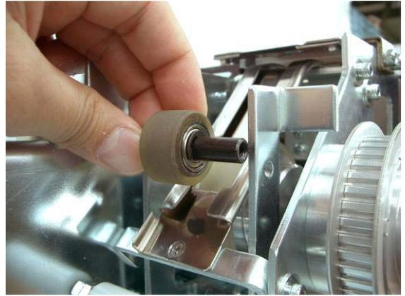
4) Dismount the E-ring so that the rubber roller can be replaced.
