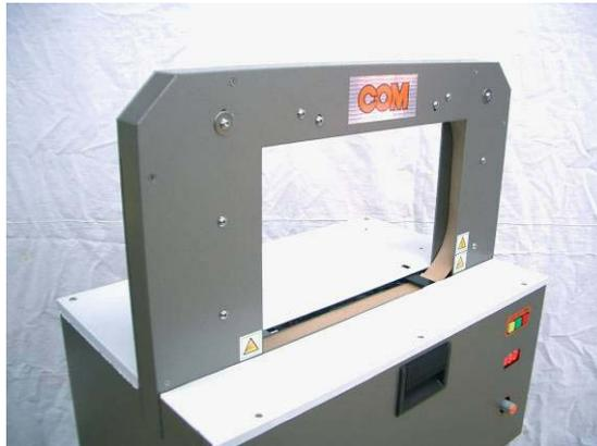
The auto sensor will be energized when the banded product is removed. The tape is then set inside the arch guide setting back the function to its origin. The machine is now ready to operate the next cycle.
